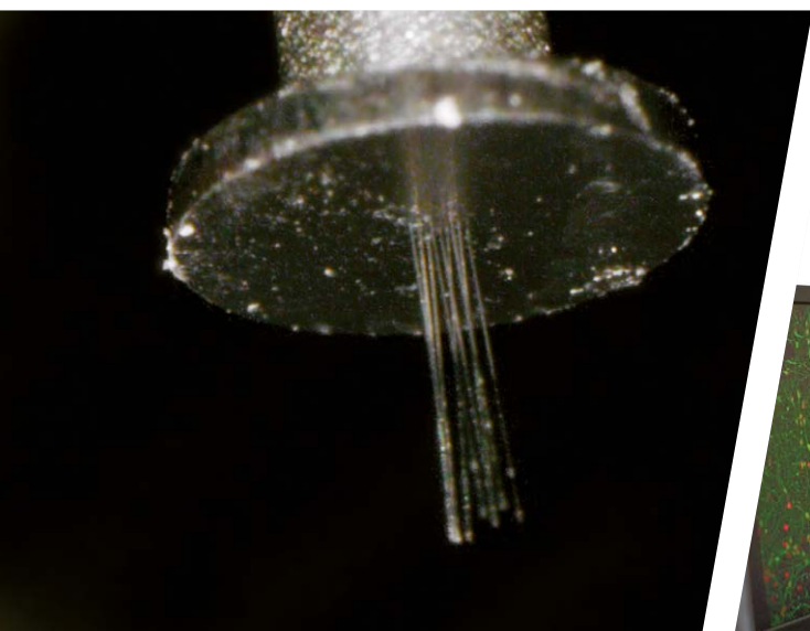
Carbon fibre penetrating electrode array, mounted on a planar base plate. The electrodes are each 8 thousandth of a millimeter in diameter.
